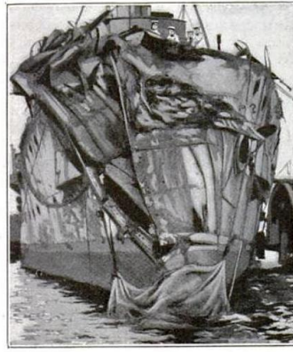
The Bow of the "Hawke," the Damage being so Great That the Ram Has Been Mashed Flat
