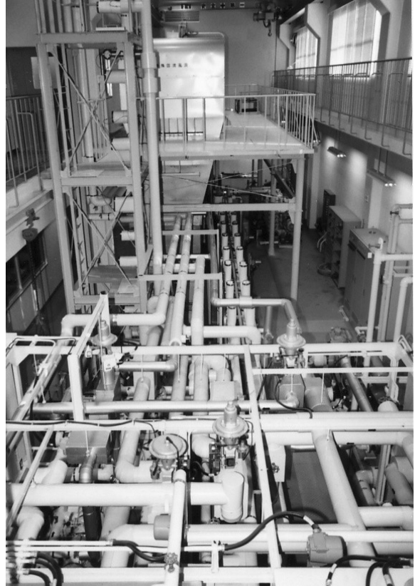
Figure 5 Experimental apparatus for developing heat pump systems using multi-component refrigerants (courtesy of Professor Koyama).
