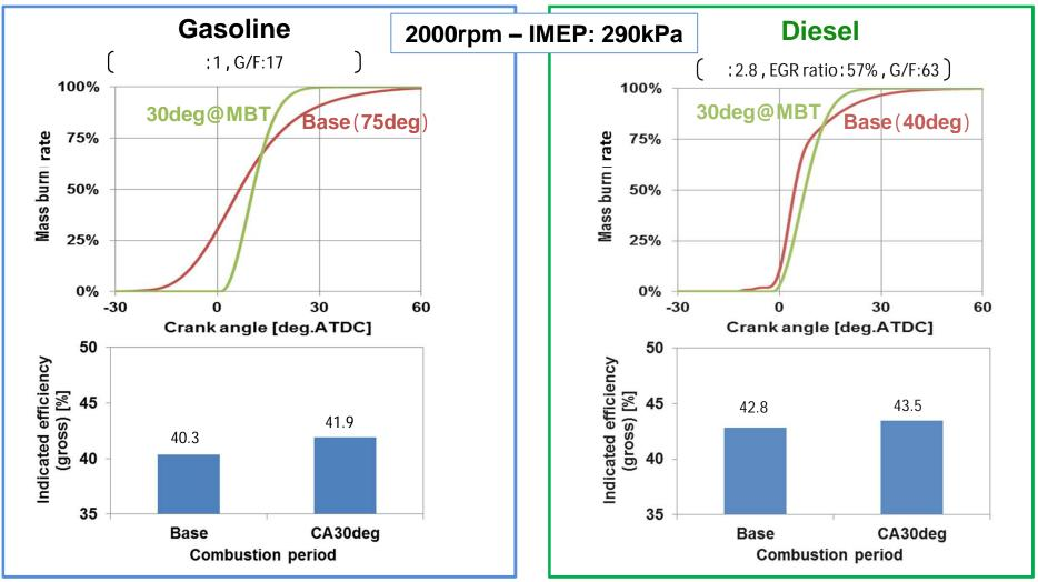
In the light load range, the effect of shortening the combustion period is two times greater in gasoline engines than in diesel engines.
