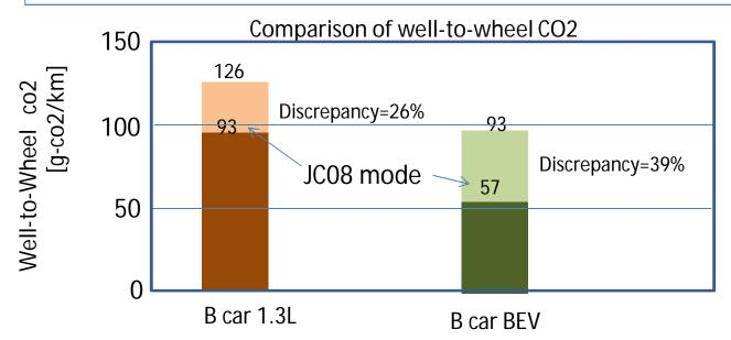
Fuel economy of internal combustion engines needs to be reduced by approx. 26%((126-93)/126=0.26) to attain the EV-level CO2 emissions.
