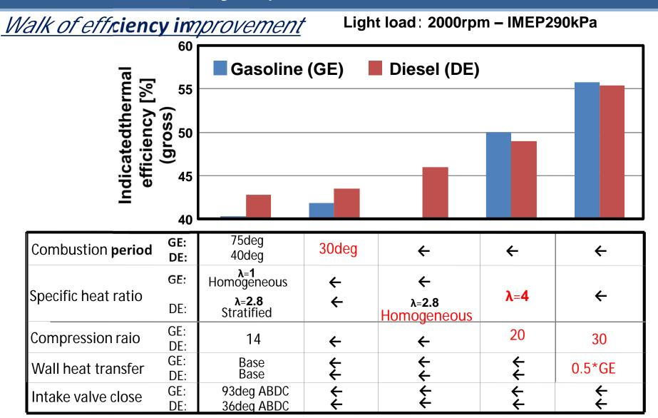
There is room for improving thermal efficiency in the light load range:Approx. 30% for diesel enginesApprox. 40% for gasoline engines
