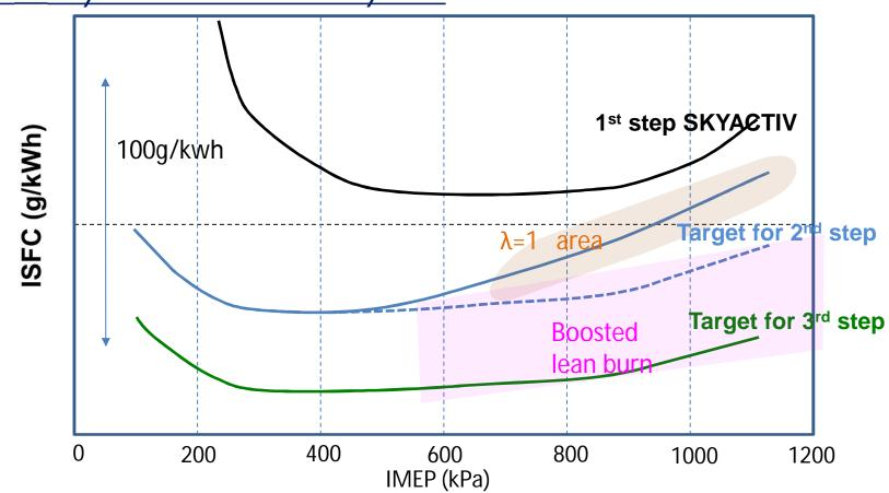
Targeted ISFC improvements Light-and-mid load: 30% in the 2<sup>nd</sup> step & 40% in the 3<sup>rd</sup> step High load rang : 10% in the 2<sup>nd</sup> step under  $\lambda = 1$ . 20% in the 2<sup>nd</sup> step & 35% in the 3<sup>rd</sup> step under boosted lean burn Will ICE vehicles catch up with EVs?
