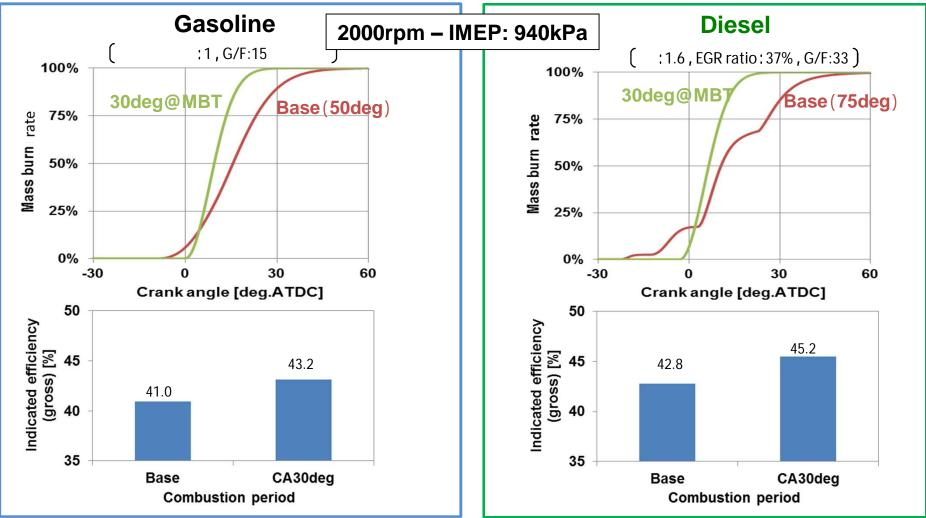
In the high load range, the effect of shortening the combustion period is almost the same between gasoline and diesel engines.
