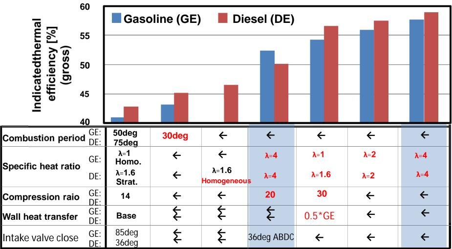
In the mid-and-high load ranges, there is room for improving thermal efficiency by approx. 40% for both the diesel and gasoline engines.
