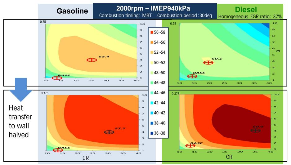
Effects of heat insulation on thermal efficiency in the high load range are almost equal to those in the light-and-mid load ranges.
