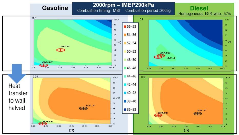
50% heat insulation improves thermal efficiency by approx. 10 % for both the gasoline and diesel engines.
