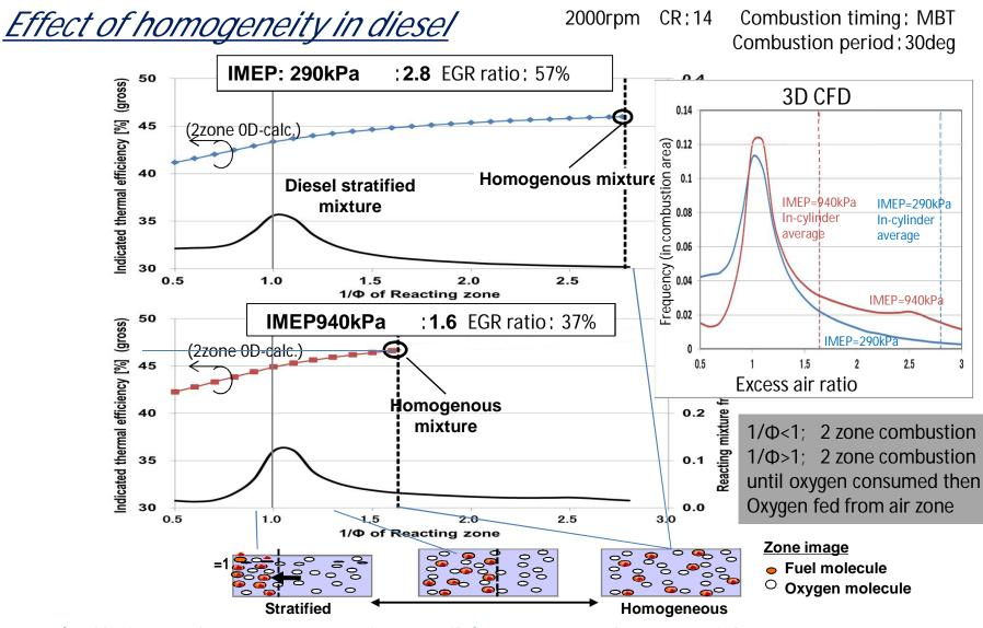
Thermal efficiency improvement is possible to some degree with an enhancement of homogeneous air and fuel mixture during fuel combustion.
